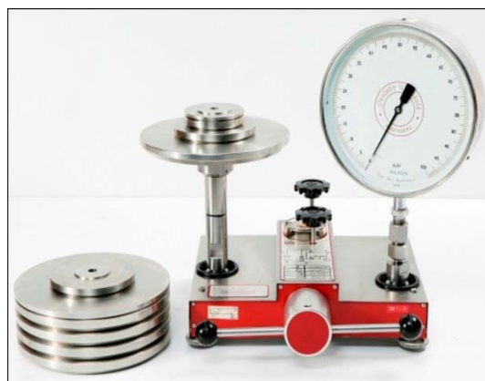
Figure 1: Dead Weight Calibrator
